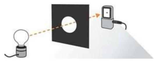
7. Press the button to measure the amount of light passing through the three holes and record '3 holes' in the text input box.
